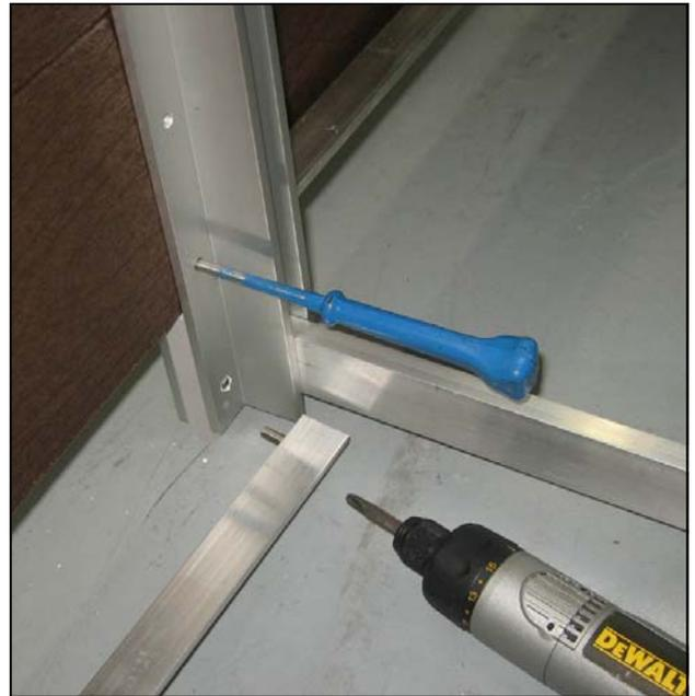
If the leg seems too tight to slide the plank in place, first check to make sure a frame screw is not impeding insertion. You may need to loosen the set screw holding a filler piece or foot in place using the supplied Allen key or Allen key bit. If it seems too tight to get the mitered plank end into the pre-assembled end panel, use the supplied 1/8" Allen key bit to loosen the set screws in the preassembled end panel a few turns.
