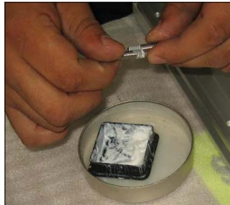
*[Note: At the factory, our method of application is to dip one screw tip into the paste and use it to spread it on a second screw (Photo above), then roll the threads together to evenly coat the tips, which will spread in the fastener hole when inserted.]*
