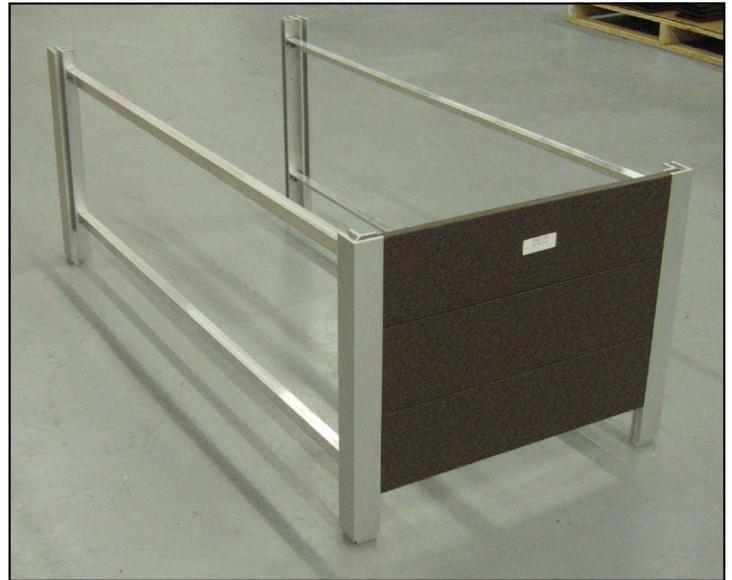
10) 1/2" x 1-1/2" x 24.5" Cross-bar mounting holes are drilled off center so that where the cross bar is used on the bottom, the hole goes down to raise the bar out of sight, and on the top piece, it goes up to lower the bar. **Photo below V**
